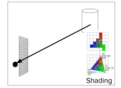
Ray Tracing Image Centric Rasterization Object Centric
